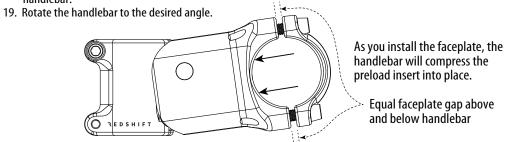
WARNING! When tightening the faceplate bolts, you are also preloading the suspension by compressing the handlebar into the preload insert. Because of this, you will notice some resistance to turning the bolts in well before the handlebar is fully clamped. It is critical to gradually tighten the bolts in an X-pattern and also to use a torque wrench to ensure you have achieved the full 5.0 N-m of torque.
