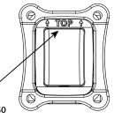
The arrows and the word "TOP" should be oriented so they are at the top of the stem.
